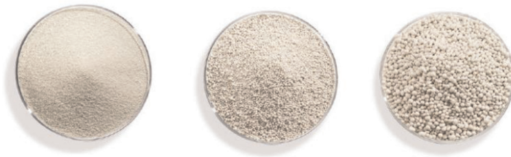
Figure 2. LWA, from left to right, Poraver 0.25–0.5, 1–2, and 2–4 mm.
