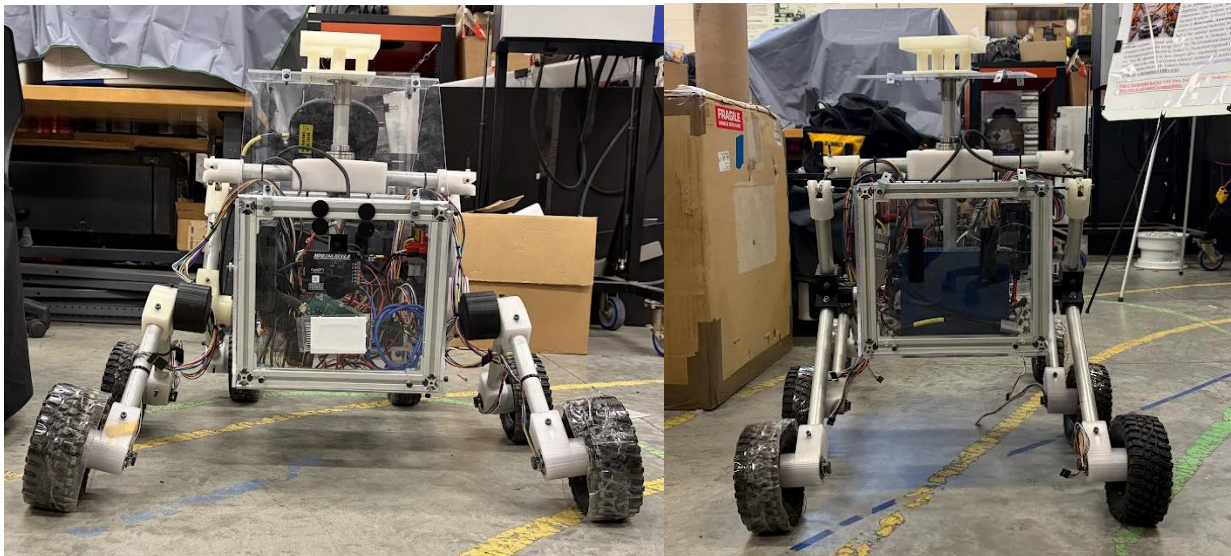
Figures 98 and 99: Existing rover showing excessive camber in suspension, and rebuilt rover with ABS prototyping joints showing camber issue resolved
