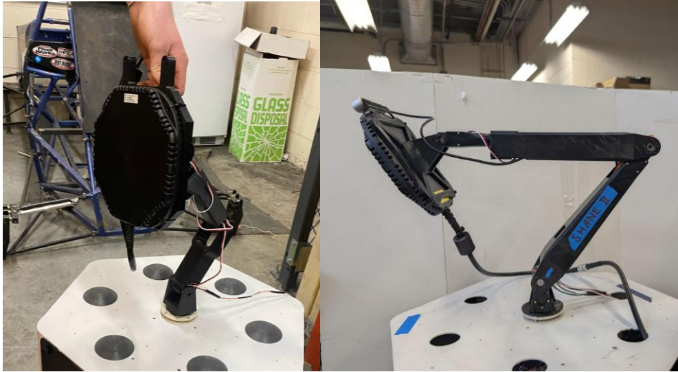
Figure 106 and 107: Gen. 1 charging station arm, and Gen. 2 charging station arm
