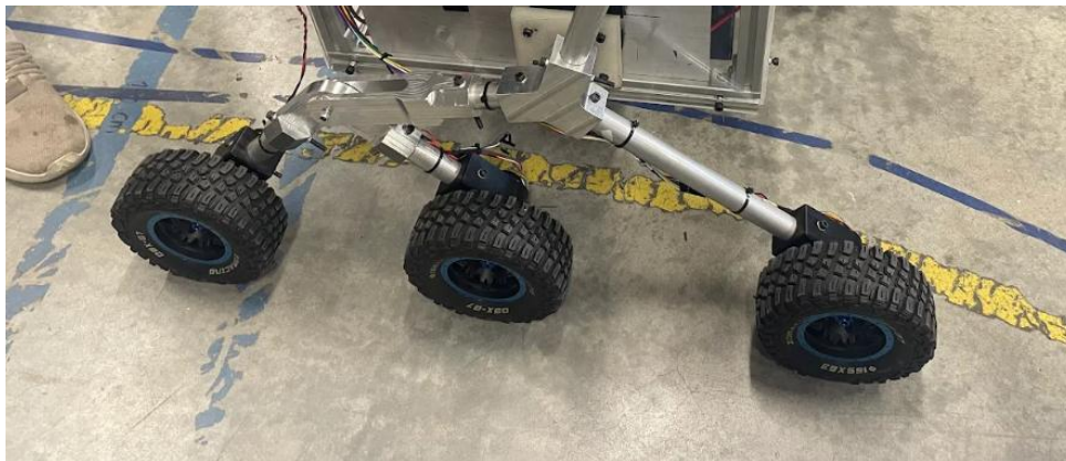
Figure 79: From left to right, rear bogie wheel, front bogie wheel, and rocker wheel
