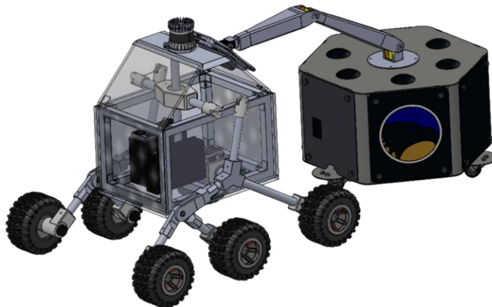
Figure 28: Full system assembly, final design
